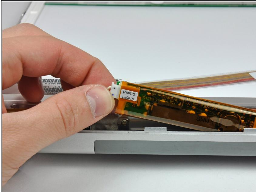
**⚠** The display inverter is a very thin and delicate circuit board that is easily broken. Use caution when handling.
