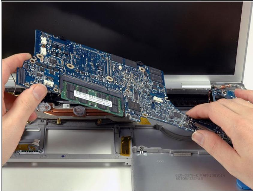
**i** The logic board is still attached to the computer by one more cable, so don't lift the logic board too far out of the computer yet.
