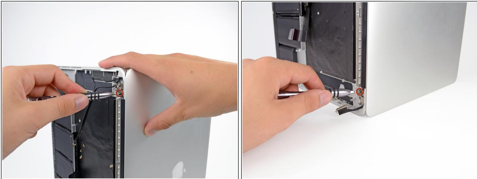
*(i)* Open the device between 90 and 100 degrees, then rest it on its side.
