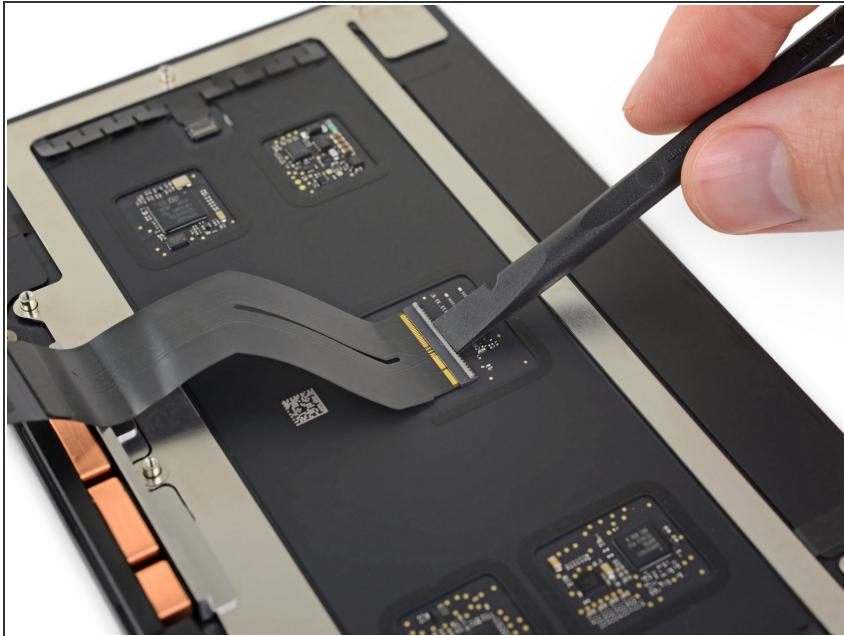
*i* If your new trackpad didn't come with a ribbon cable, use the following three steps to remove and transfer the old ribbon cable to the new trackpad.
