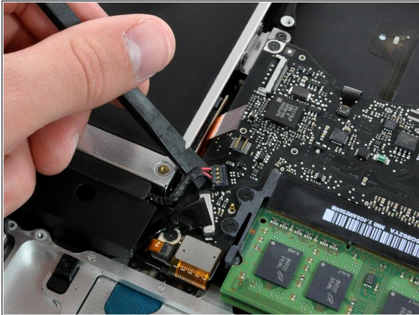
**i** If necessary, peel off the foam bumper covering the subwoofer connector.
