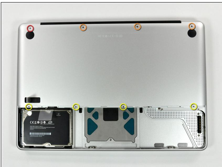
Remove the following eight screws securing the lower case to the chassis:
