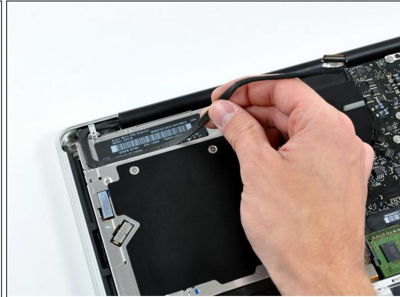
*(i)* If necessary, peel the EMI gasket off the camera cable connector.
