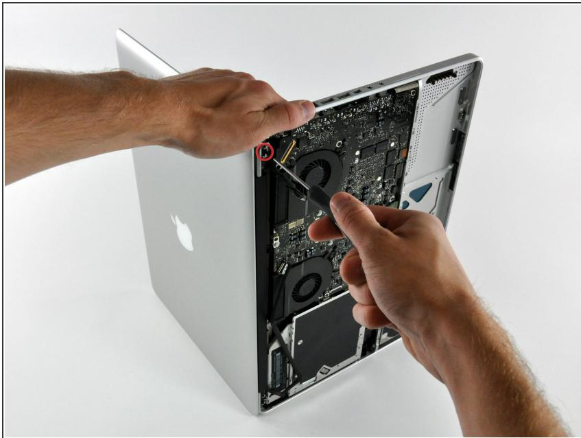
**⚠** Be sure to hold the display and upper case together with your other hand. Failure to do so may cause the freed display/upper case to fall, potentially damaging each component.
