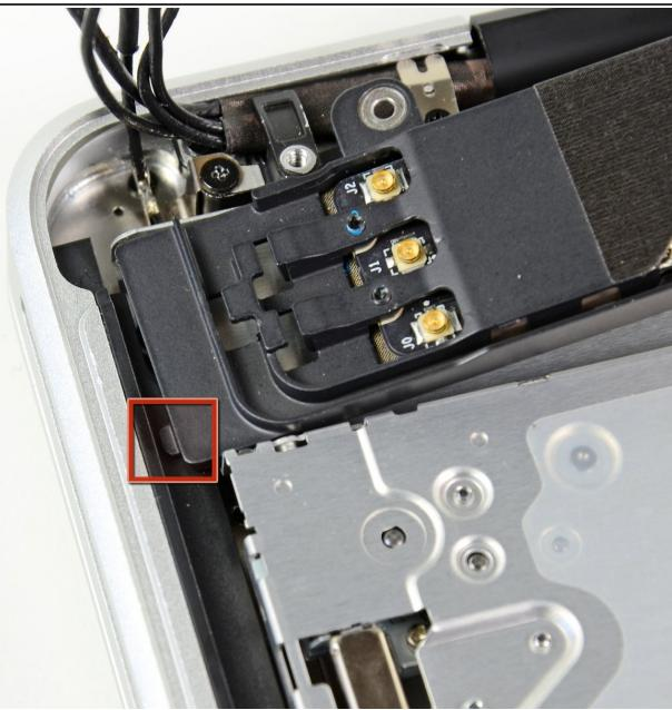
Before securing the AirPort/Bluetooth bracket to the upper case, be sure the small tab on its left edge is inserted into the small void cut into the black plastic optical drive opening.
