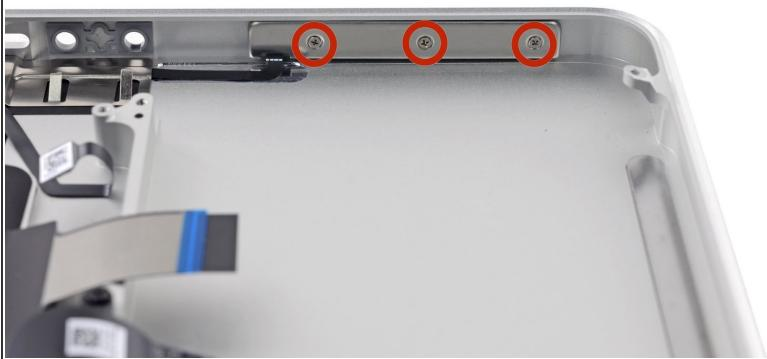
**i** Before proceeding, check if your replacement upper case comes with the battery level indicator installed. If not, you'll need to transfer the battery level indicator to your new upper case.
