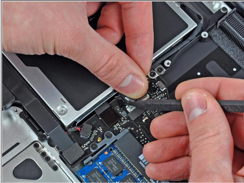
**i** The camera cable connector is not secured by any locking or snapping mechanism. Hence, Apple sticks a small strip of black plastic with adhesive applied to the side facing the logic board behind the camera cable connector to keep it in its socket.
