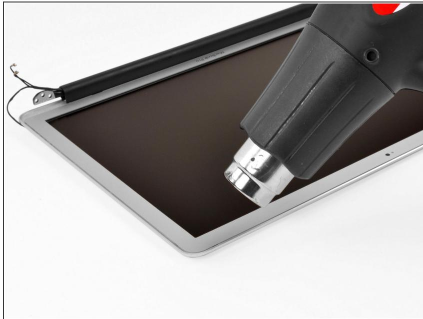
**i** In the following steps, you will use a heat gun to soften the adhesive securing the outer silver border around the underside of the front panel to the display.
