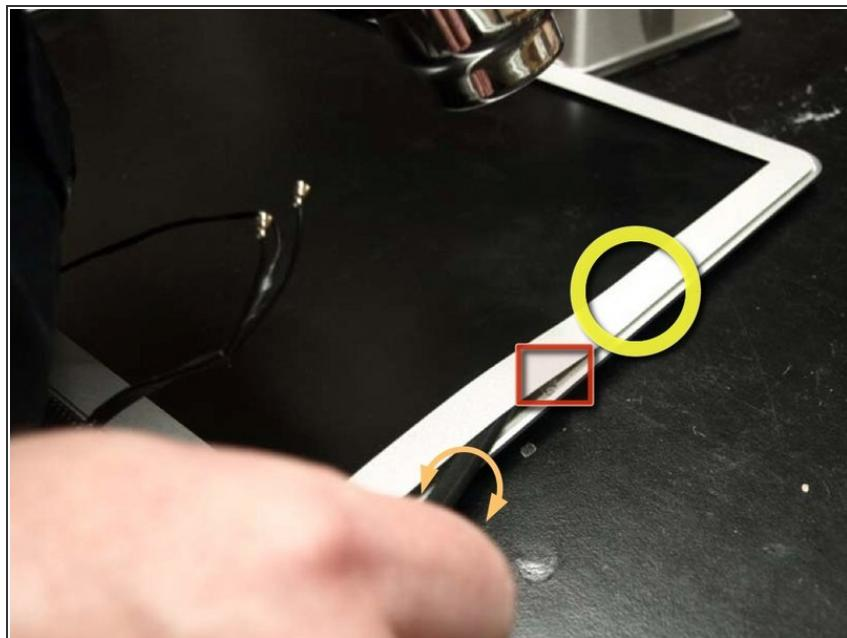
**⚠** Only insert the spudger from the outer edge of the display assembly, and do not push it more than 6mm (1/4in) towards the inner edge of the bezel - otherwise you risk damaging a gasket between the inner edge of the bezel and the screen.
