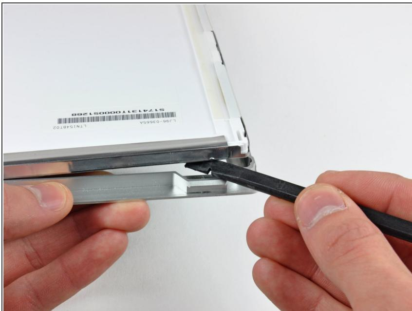
**i** The next few steps will require you to separate the LCD from the adhesive applied to the upper and lower edges of the front bezel.
