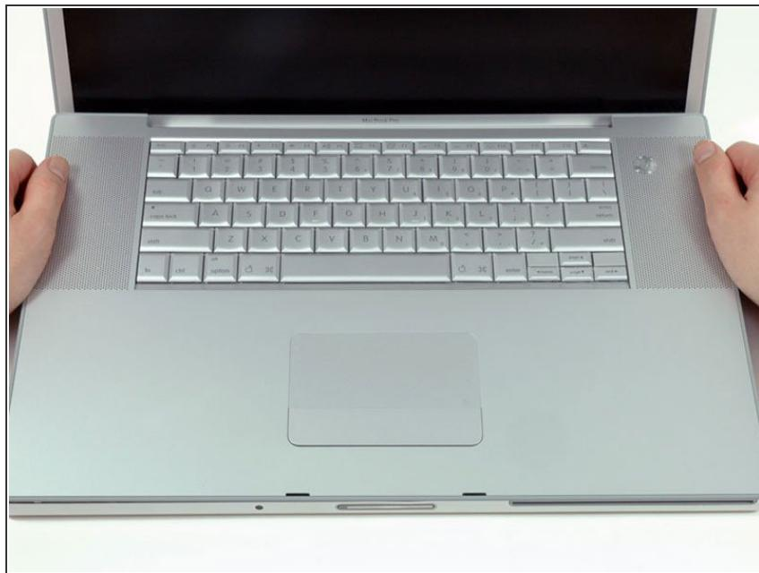
**⚠** Do not yank the upper case off quickly. The case is attached to the logic board via a ribbon cable.
