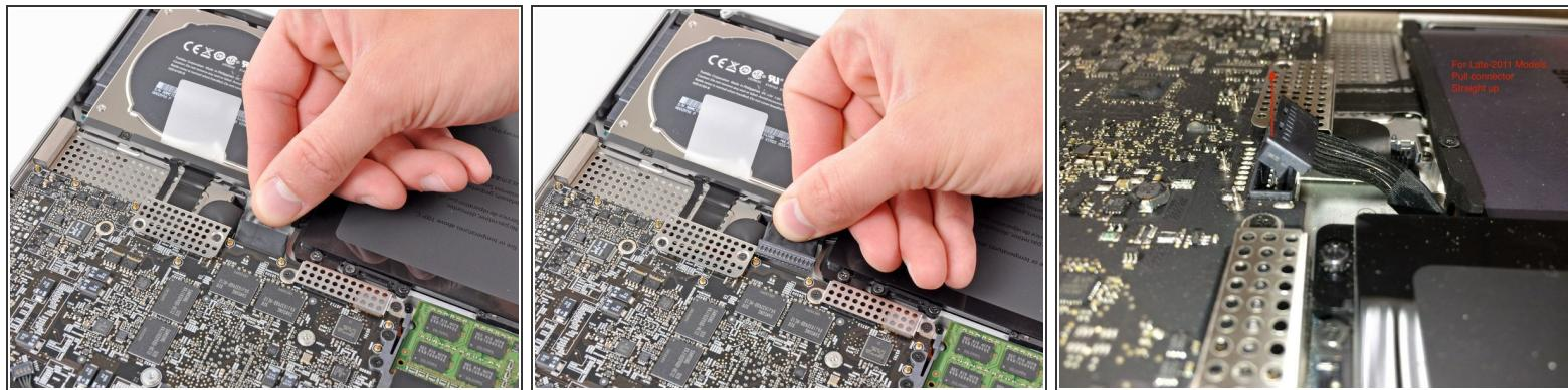
**⚠** Whenever working near the logic board, it is always wise to first disconnect the battery to avoid short circuits.
