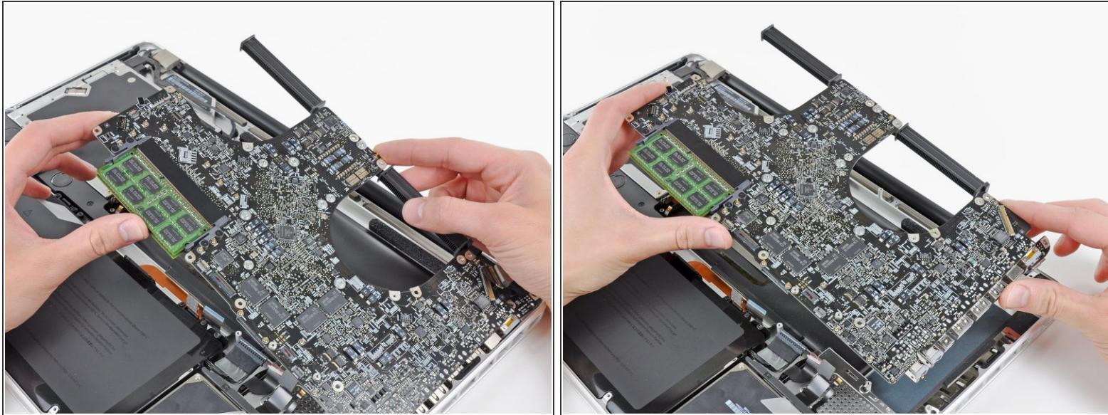
⚠ Handle the logic board assembly by its edges only.
