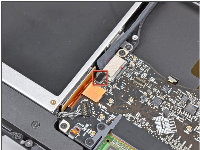
i Before disconnecting the camera cable, a small plastic retainer stuck to the logic board must first be moved out of the way.
