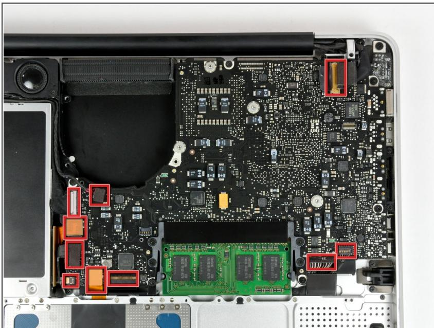
*(i)* In the next few steps, you will disconnect the highlighted cables which connect the logic board to the upper case.
