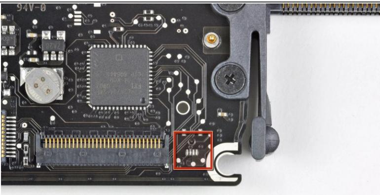
**⚠** Some 2.0 GHz A1278 MacBook Unibody logic boards do not have the necessary socket installed to accept the keyboard backlight ribbon cable attached to the upper case. The first and second pictures show logic boards with and without the socket installed, respectively. If your logic board does not have the backlight ribbon cable socket installed, the keyboard **will** work but the keys **will not** light up.
