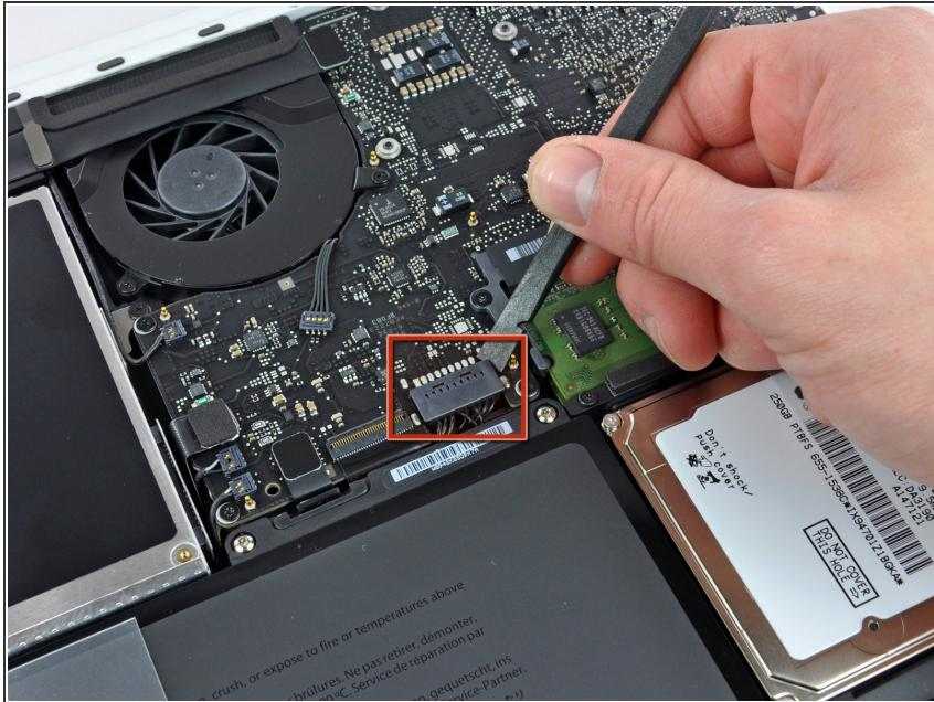
**⚠** For precautionary purposes, we advise that you disconnect the battery connector from the logic board to avoid any electrical discharge. This step is **optional** and is not required.
