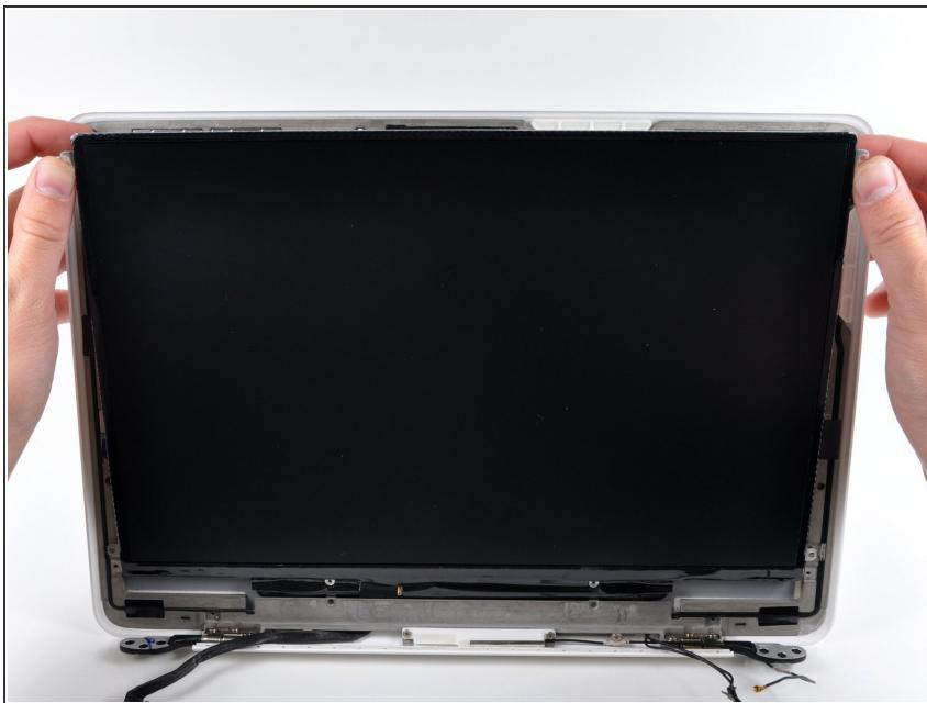
**⚠** Do not try to remove the LCD yet. The circuitry along its lower edge is wedged in a gap along the lower edge of the display recess in the plastic display assembly.
