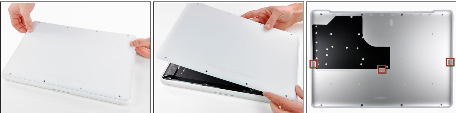
**⚠** The lower case is constructed of rubber-coated aluminum. Do not excessively bend the aluminum during removal, as any permanent deformation will cause tolerance issues after reassembly.
