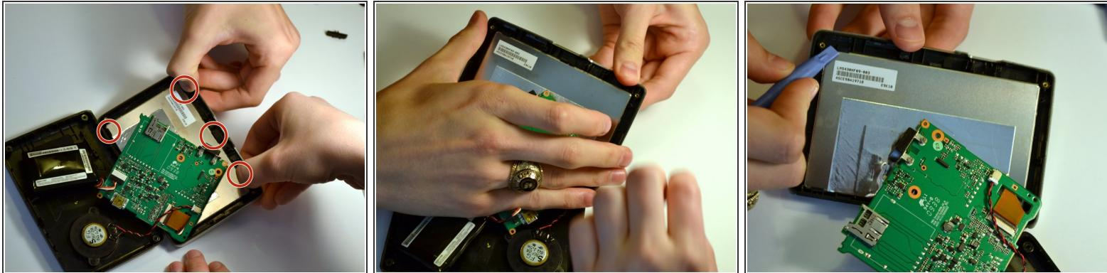
*(i)* It may be necessary to get help from a friend to hold the device stable while removing the screen.
