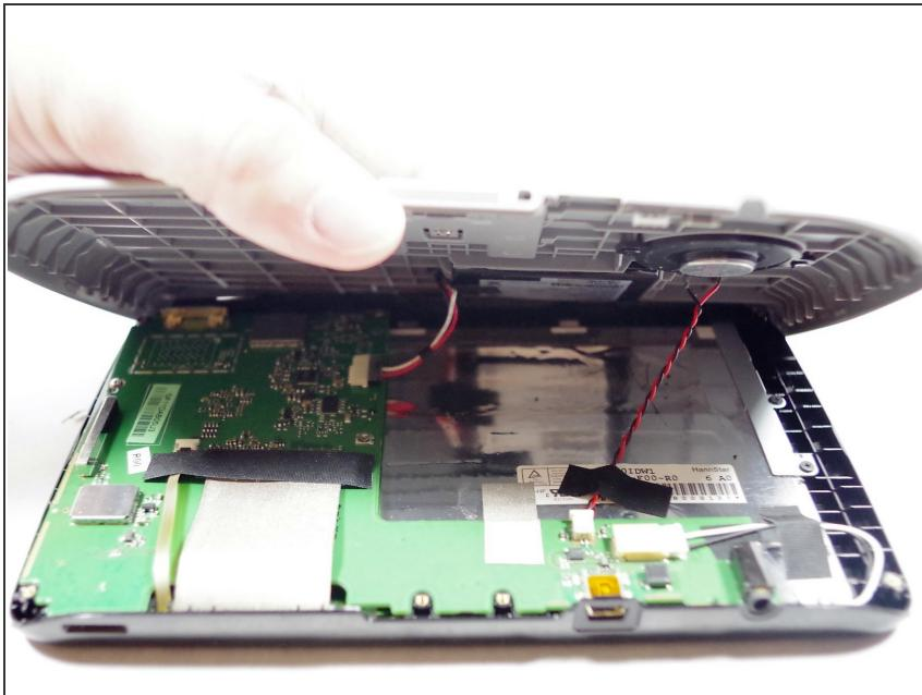
**⚠** Lifting the back panel too quickly or forcefully may damage the speaker cable and battery cable, which are still attached underneath.
