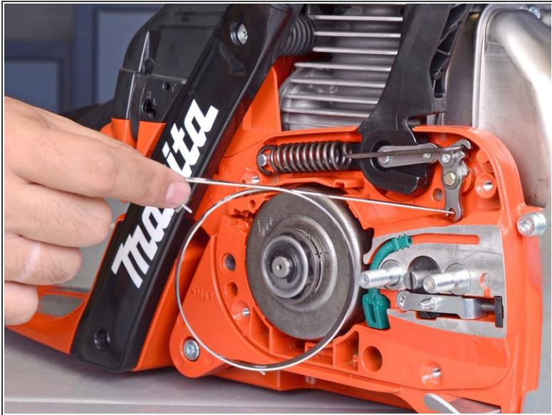
**⚠** From this point forward, be careful not to engage the chain brake. If the brake snaps back into the locked position during repairs, it may pop the stiff tension spring out of place. You can tie the guard handle to the tube handle with some string as a precaution.
