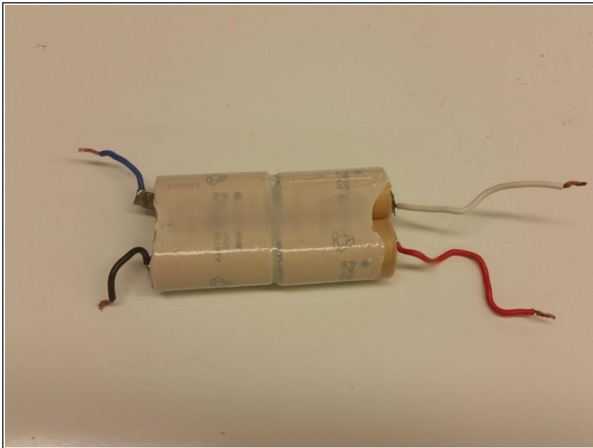
*(i)* The drill uses a battery pack consisting of four NiCd cells each with a nominal voltage of 1.2V. This gives a total pack voltage of 4.8V when all batteries are connected in series.
