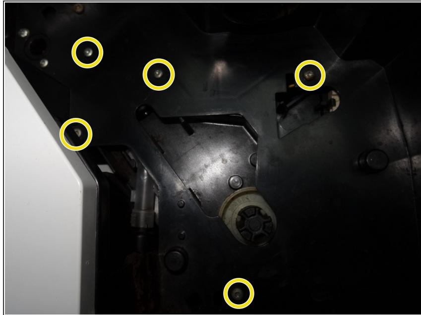
*i* The drainage valve is directly plugged to the gear drive. The drive is fixed with five Torx T10 screws on the center panel behind the brew group.
