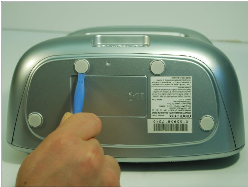
**(i) The bottom panel screws and screw covers must be removed in order to access the back panel.**
