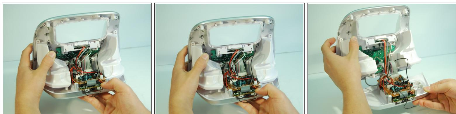
! Be careful when removing the bottom panel. The plastic tab that runs alongside the right speaker between the upper brown radio motherboard and the lower green audio daughterboard may damage the device if the bottom panel is removed improperly.
