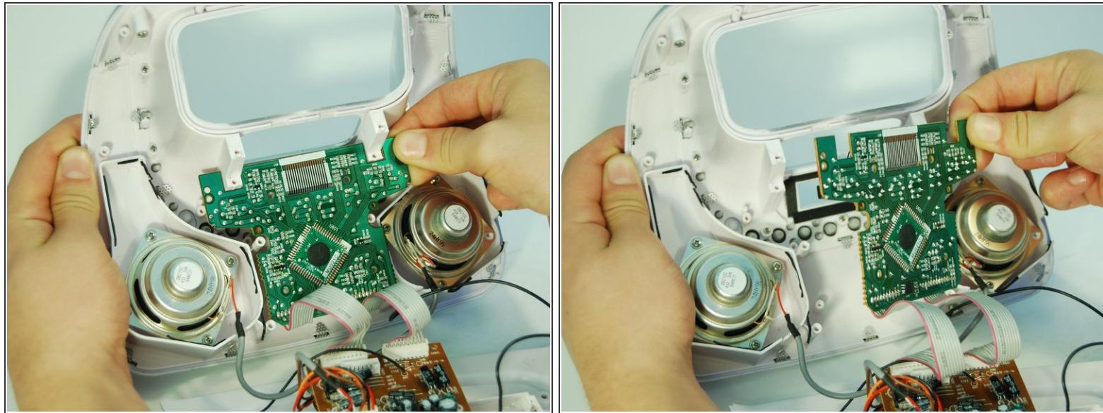
**⚠** Be careful when removing the daughterboard. There are still two wires connecting the display daughterboard to the radio motherboard which can be damaged or ripped if recklessly removed.
