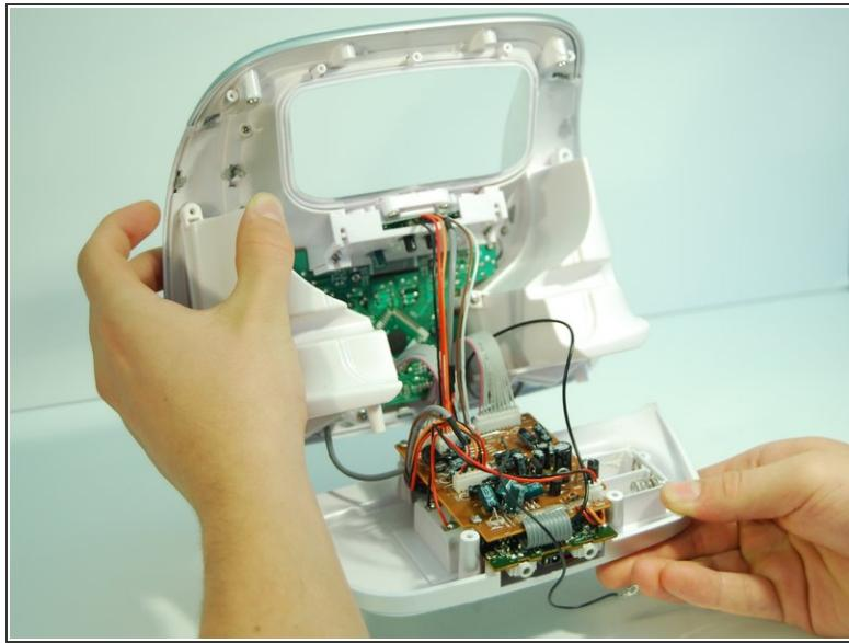
**⚠** A plastic sheet is in between the radio motherboard (the upper brown board) and the audio port daughterboard (the lower green board) coming from the right speaker housing. Be careful when removing the back panel as to not damage the boards.
