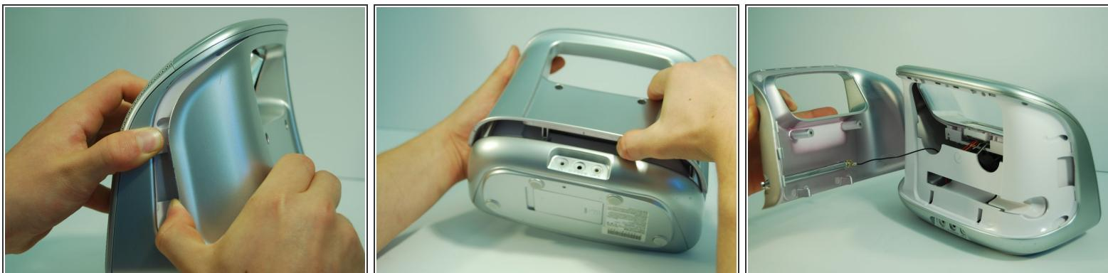
! Be careful not to use too much force to remove the panel. The antenna wire is connected to the inside of the panel and may be damaged or ripped off if the panel is not gently removed.
