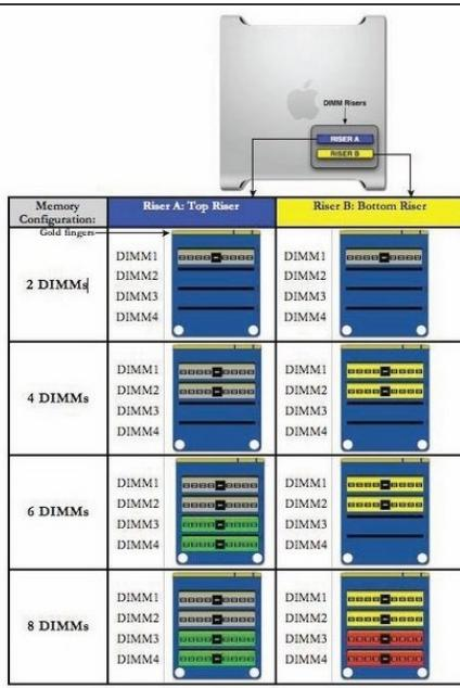
**i** Additional pairs of 1 GB, 2 GB, or 4 GB FB-DIMMs can be installed in the open DIMM slots. Maximum memory is 32 GB.
