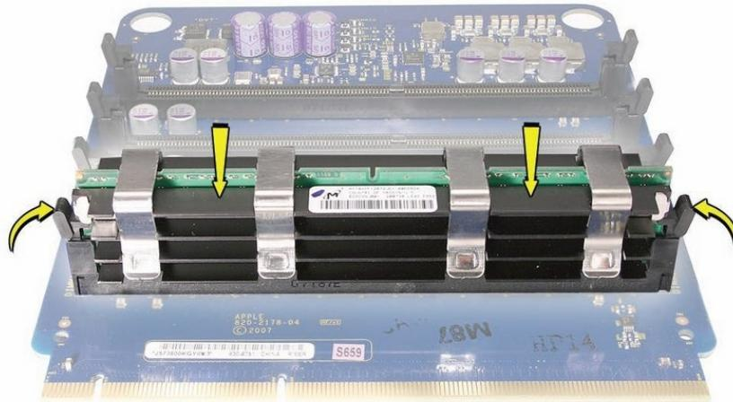
**i** Replacement Note: Align the DIMM in the slot on the riser card and push both ends of the DIMM down until the ejectors snap back up into place.
