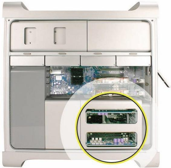
**!** Warning: Always wait 5–10 minutes for the computer to cool down before you remove or install memory. The DIMMs may be very hot.
