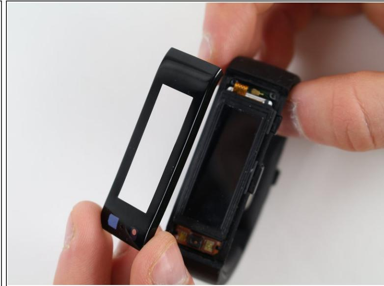
**⚠** Do not pull the frame away too quickly. The screen may be stuck to the frame, and pulling on it could cause damage. If the screen is still attached, lightly push on the screen with a finger and it should pop out.
