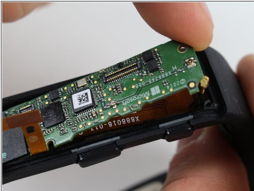
⚠ Be gentle. Make sure not to rip apart the cord underneath that connects the heart-rate monitor to the motherboard.
