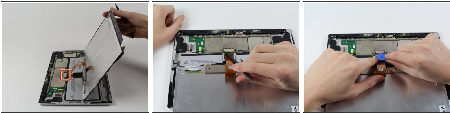
**⚠** The RF shield that you are about to remove will be damaged in the process. you may be able to bend it back into shape once you remove it.
