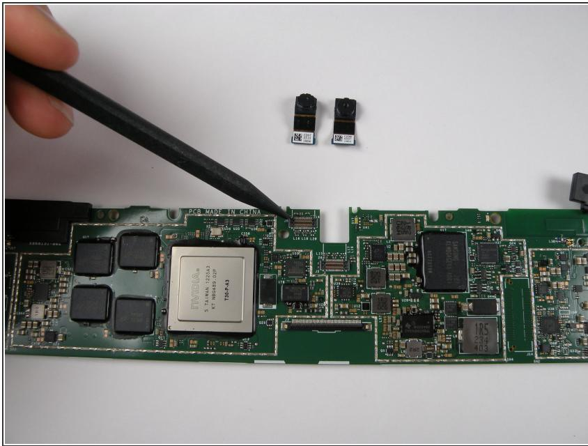
When you replace the camera(s), and make sure that they line up with the front and back cover.
