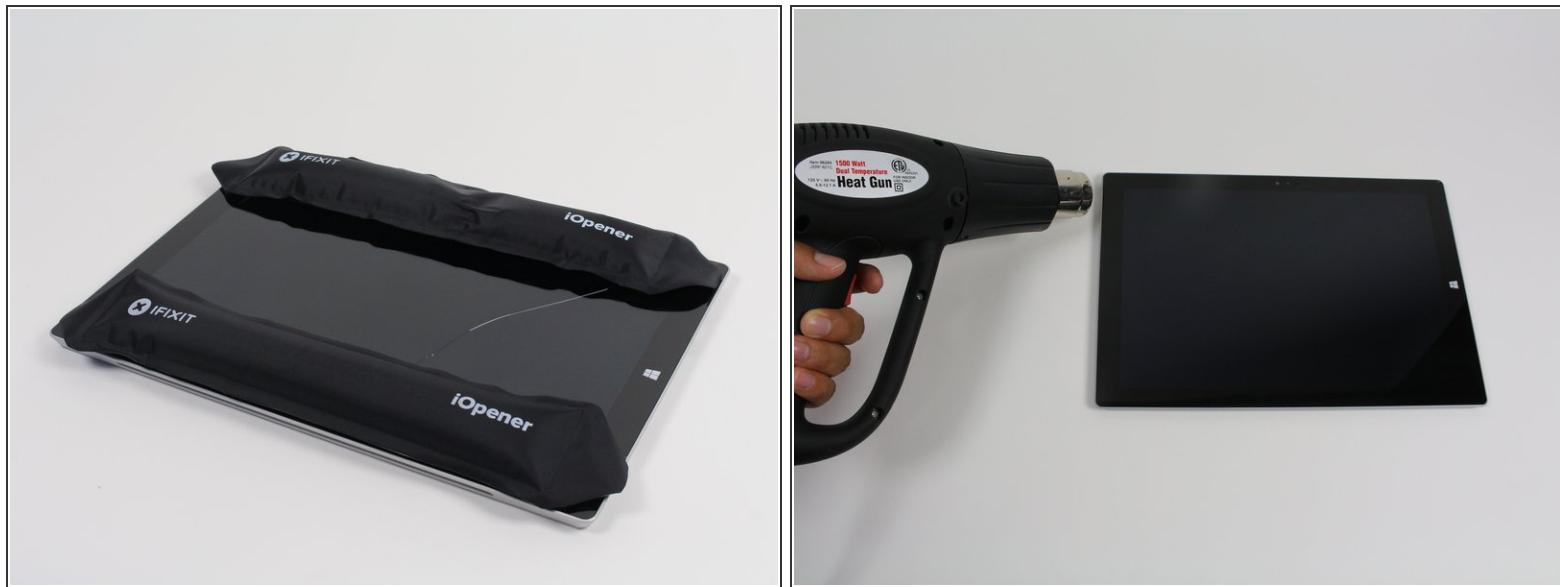
**⚠** Before you begin, discharge the Surface Pro's battery below 25%. A charged lithium-ion battery can catch fire and/or explode if accidentally damaged during the repair.
