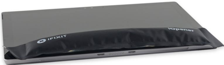
**i** The display is strongly glued to the frame of the device.
