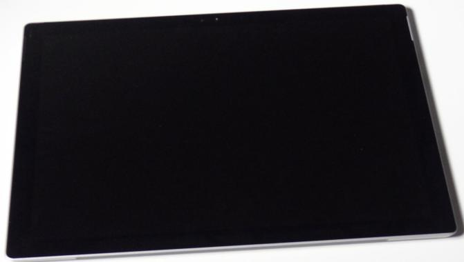
**⚠** Before you begin, discharge the Surface Pro's battery below 25%. A charged lithium-ion battery can catch fire and/or explode if accidentally damaged during the repair.
