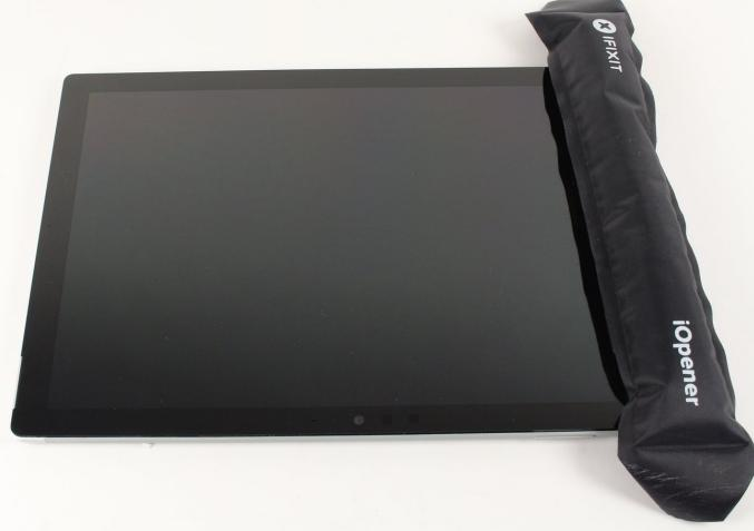
**⚠** Before you begin, discharge the Surface Pro's battery below 25%. A charged lithium-ion battery can catch fire and/or explode if accidentally damaged during the repair.
