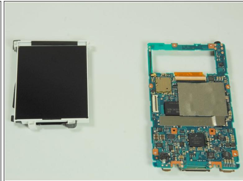
*(i)* The LCD ribbon cable is clamped in place.
