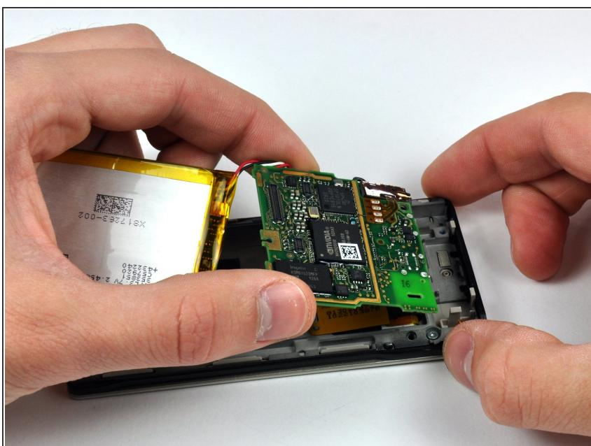
*i* For this step, it is recommended to cautiously hold the battery and logic board assembly with one hand while holding the inner chassis with the other.
