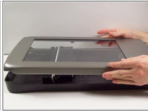
⚠ Do not fully remove the lid until you remove the ribbon cable attached to the front of the upper lid.
