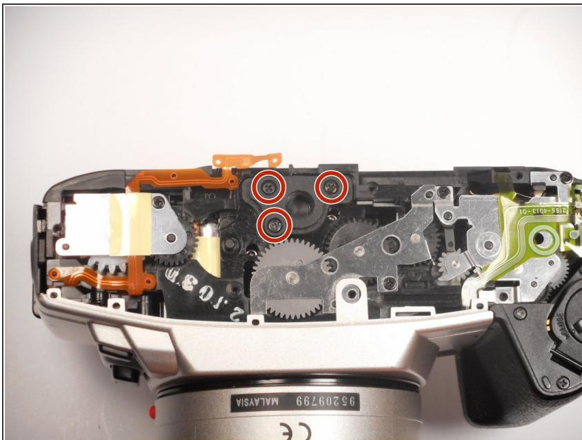
**i** The tripod socket is visible when the bottom panel is removed.
