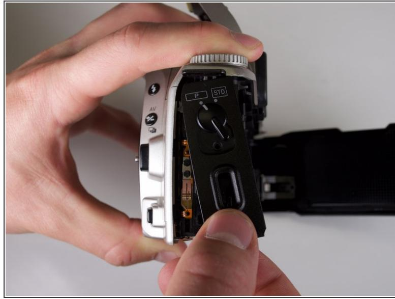
**⚠** Be careful when removing the right side panel. There is a plastic component underneath the side panel that will come free. Note the orientation of this plastic component for reassembly because it is connected to the back-cover release switch.
