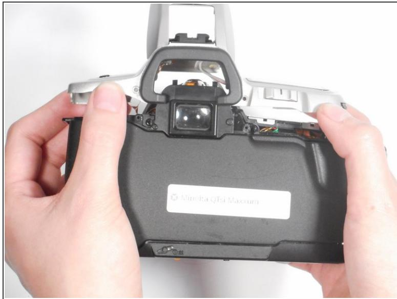
**i** The top panel of the camera should now be easy to lift off. If it is not, make sure that all screws and attachments, listed in steps 1-5, have been removed.
