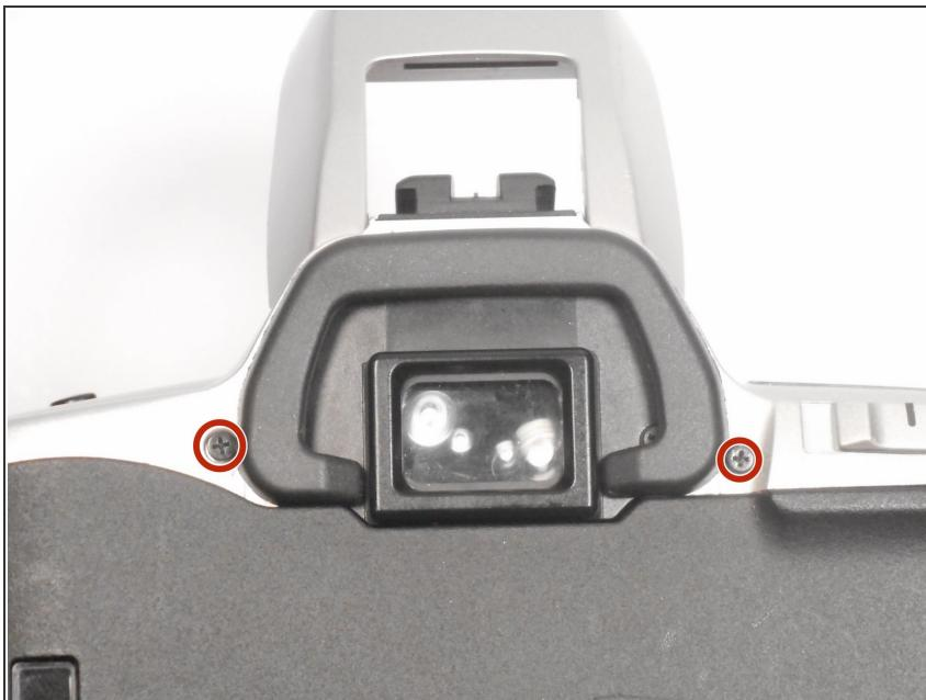
**i** The only screws remaining that hold the top panel of the camera in place are located next to the view finder.
