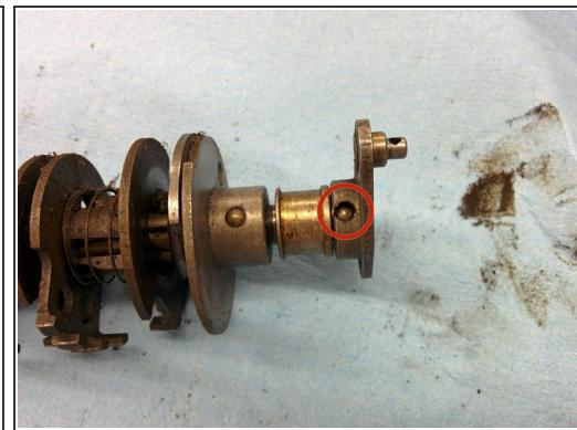
*(i)* It's called that because when you press a key, rock bars cause the plates on the assembly to move so that the same number of teeth as the key you pressed will be selected to engage other gears.
