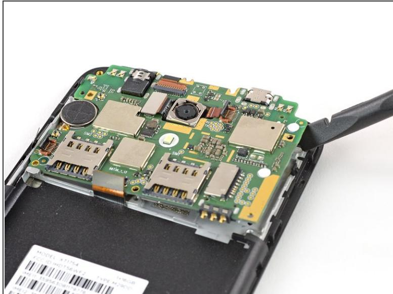
! Don't try to remove the motherboard all the way yet. The antenna cable is still connected to its rear side.
