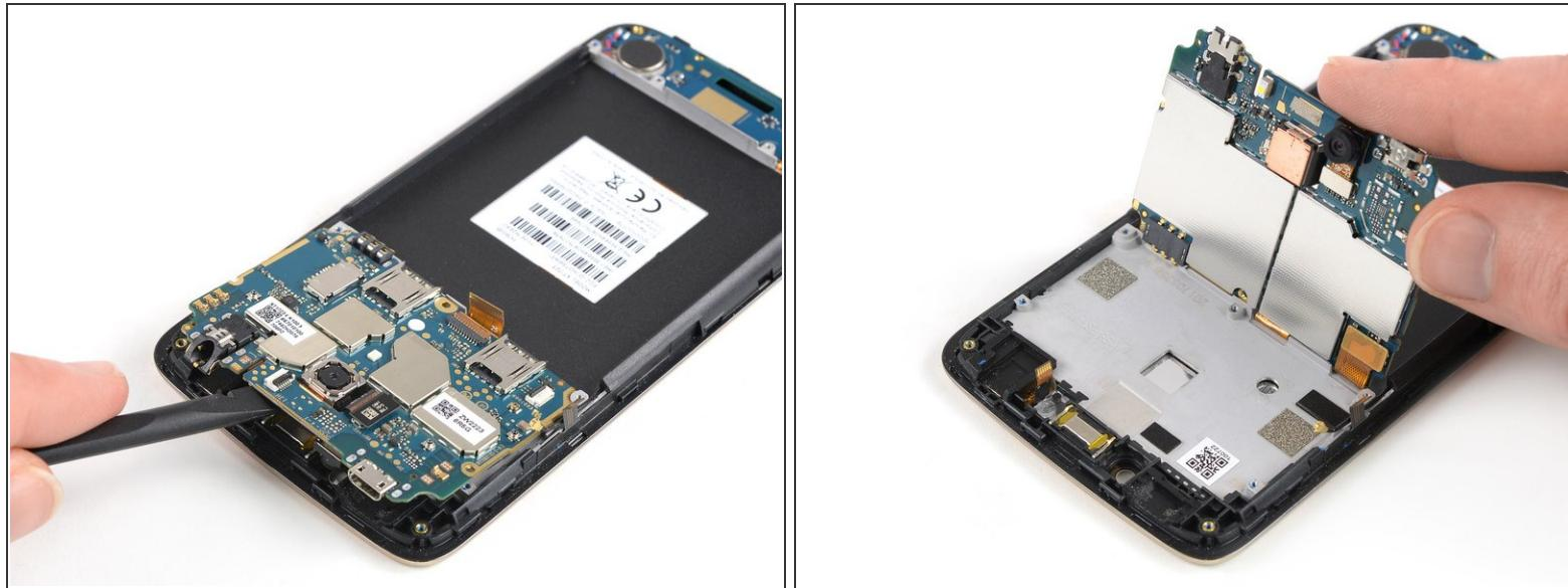
⚠ Don't try to remove the motherboard all the way yet. The display flex cable is still connected to its rear side.
