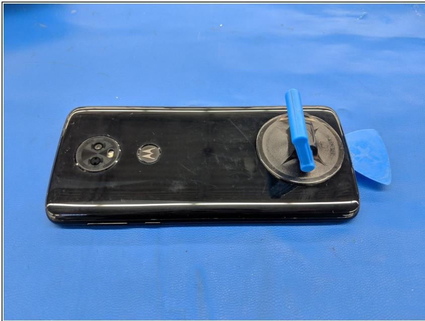
! The back and frame of this phone is made of plastic. Be careful when heating the phone.
