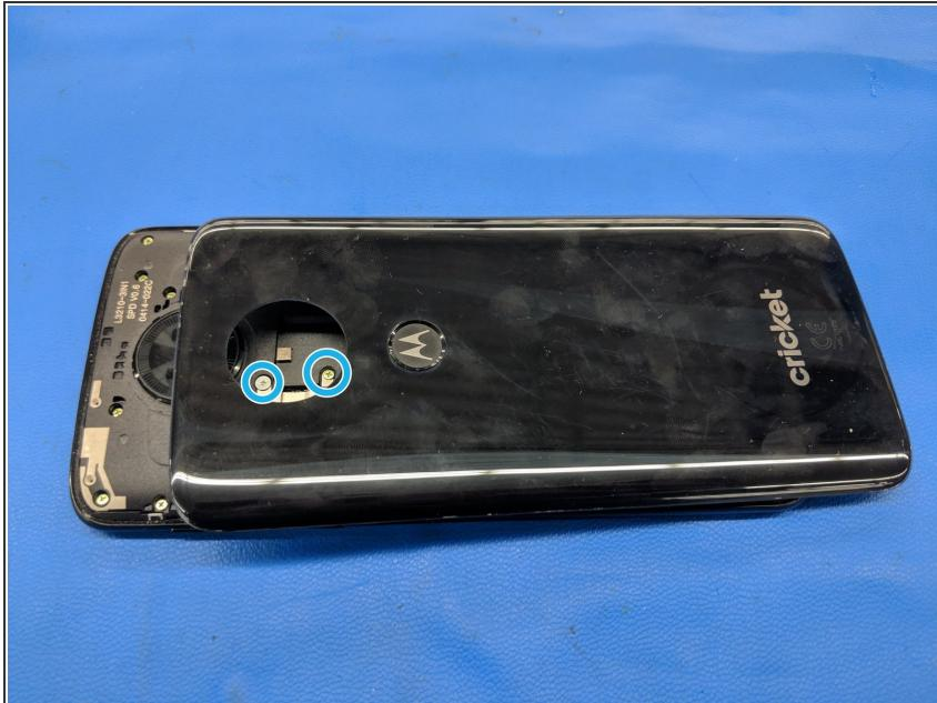
! The back of the phone is still attached via the fingerprint sensor's ribbon cable.
