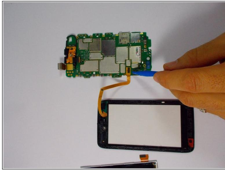
**⚠** Remove the ribbon cable connecting the LCD display to the motherboard, be mindful that the ribbon cable is very thin.
