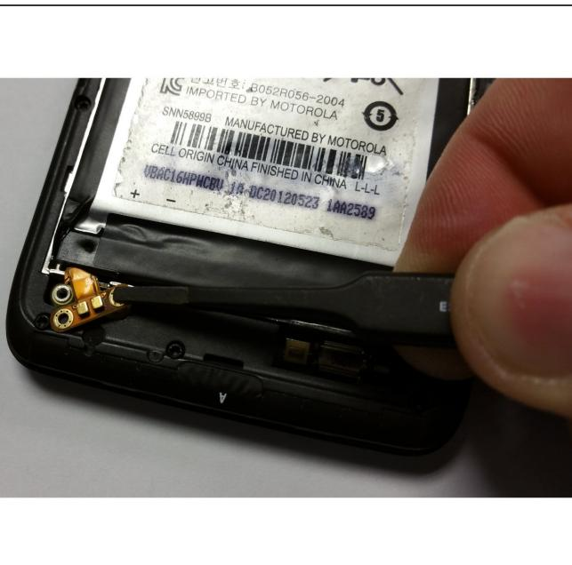
⚠ Lift the battery leads to the upward position. The ribbon cable is very thin, be gentle.
