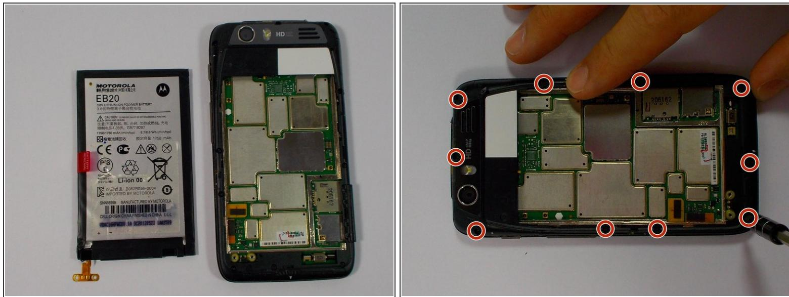
*(i)* The back case portion may be removed after the battery has been removed.
